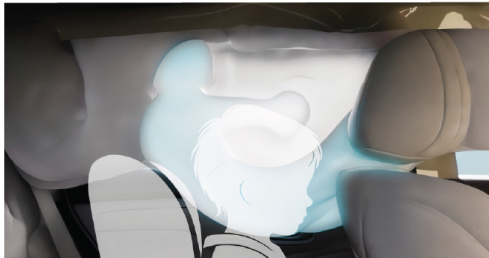
Extra-long Side Curtain Airbag 2.1-meter extra-long side curtain airbags with rollover protection, instantly and preemptively deploying upon rollover to provide comprehensive occupant protection.
