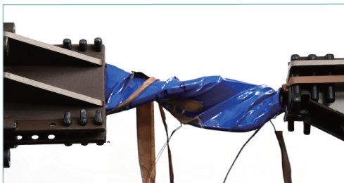
Magazine Battery 2.0 Enhanced battery performance and elevated safety standards, with fully charged battery enduring a 180-degree twist without catching fire.
